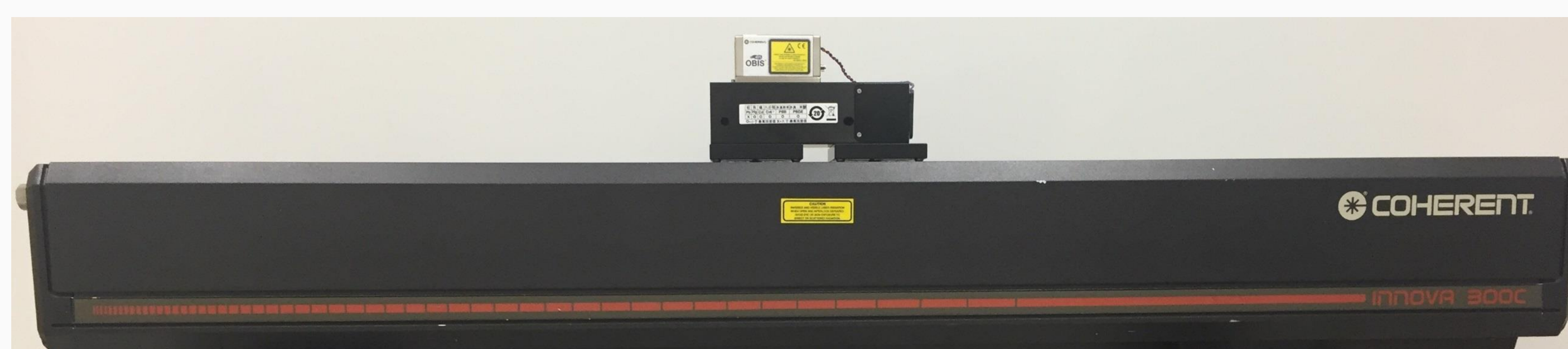
Figure 4. Size comparison of the original laser and its replacement with heat sink.
